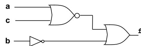
d) Construct the truth table describing the output of the following circuit and write the simplified Boolean equation (6 pts).
